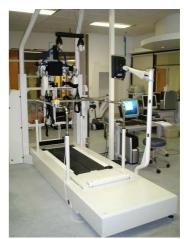
Installed in a pit, Belts and floor at the same level Here connected to a motion analysis system VICON.
